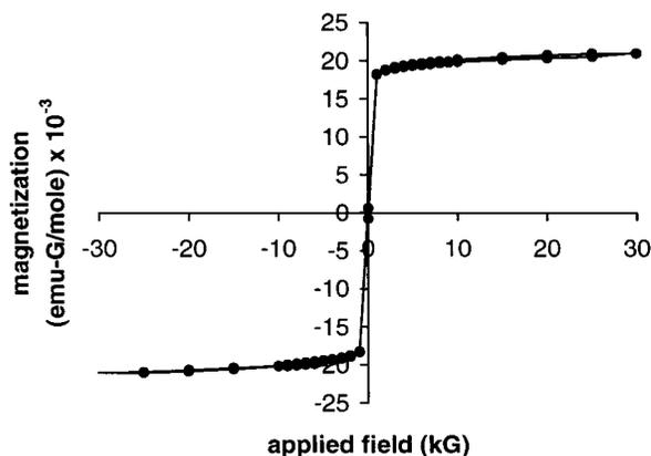
**Figure 6.** Plot of magnetization vs applied field at 1.8 K for  $[\text{Cr}(\text{Cp}^*)_2][\text{DMeDCF}]$ .
