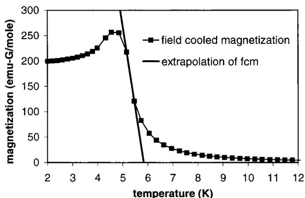
**Figure 4.** Plot of magnetization vs temperature in 2 G applied field for  $[\text{Cr}(\text{Cp}^*)_2][\text{DMeDCF}]$ .
